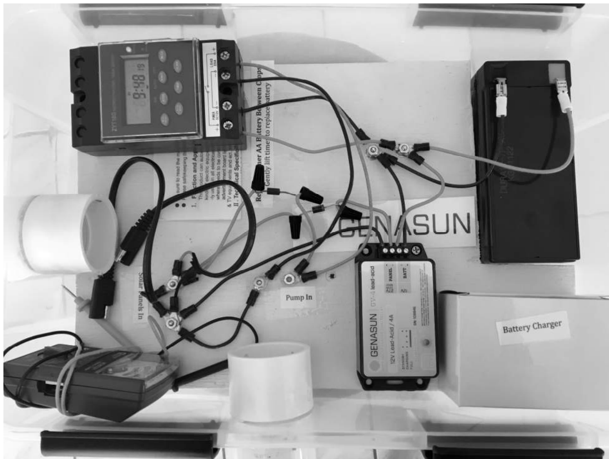
Figure 24 Electrical box. Contents include battery (12v, 7ahr); Genasun solar charge controller; programmable timer (instructions beneath); battery charger; and battery tester (green). Solar panel inputs enter through the elbow on the left and mate with the connectors at “solar panels in”. Pump wires enter through the elbow at bottom of picture and attach to the terminals labeled “pump in”. Pump brown (+) and black (-) wires connect with circuit red (+) and blue (-) wires respectively. Everything is easy to reach especially the timer for programming. Lift the timer to access the single AA battery that we recommend changing between crops. The battery charger is for emergency charging only as in operation the battery stays continually charged by the solar panels. The battery tester is useful for measuring solar panel input as well as battery current.
