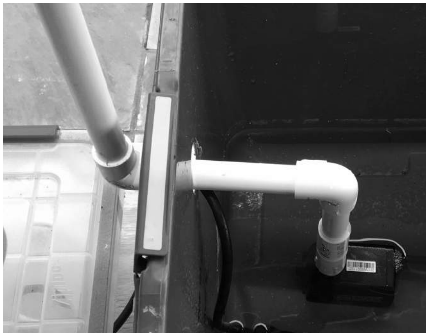
Figure 18. Note the connection between the pump and the drip irrigation system.
