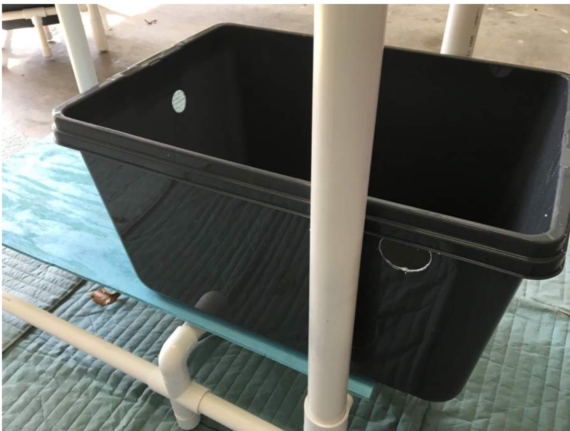
Figure 12. Reservoir positioned correctly on the reservoir support board
