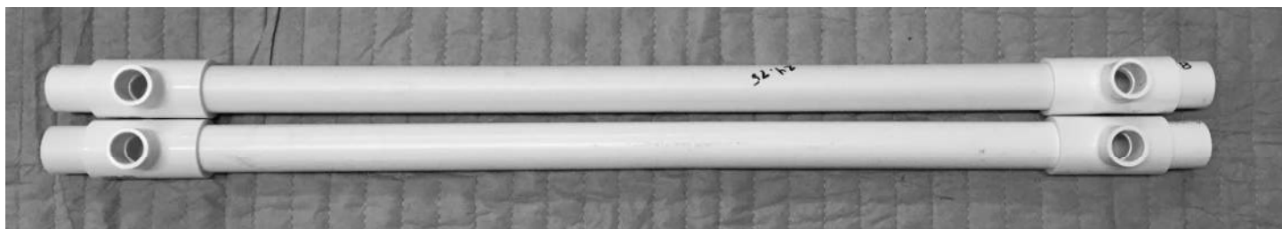
Figure 5. The top side bars. The tees are reducing tees that will support an optional ½" Frost Protection Overhead Rack
