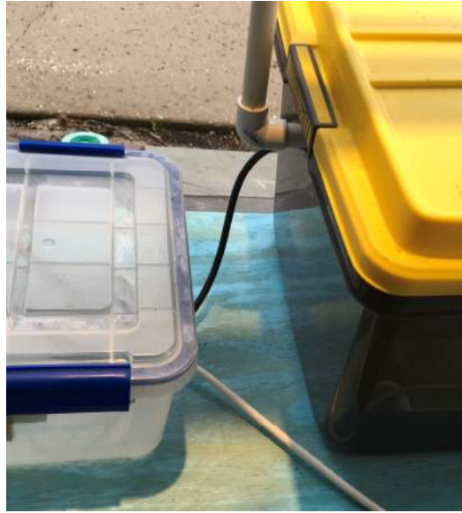
Figure 19. The pump (black) and lamp (white) cords enter the electrical box.
