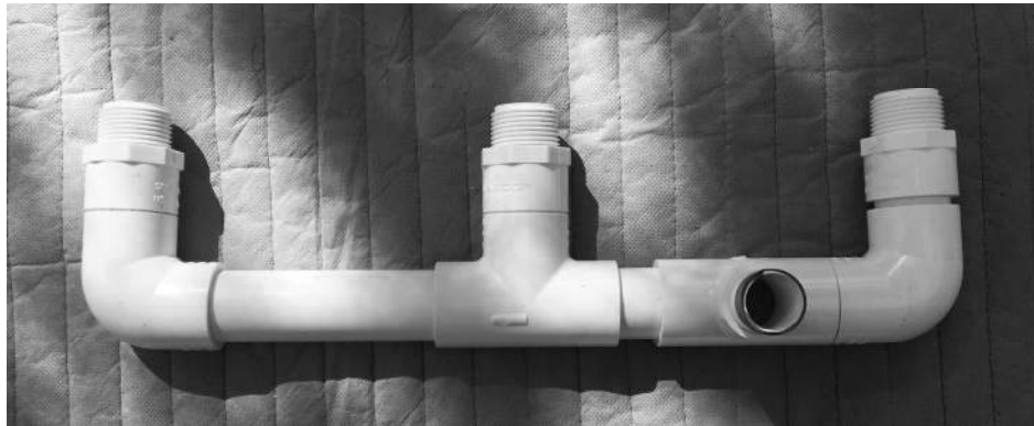
Figure 10. The manifold, shown upside down (In its operating position the open tee points down and to the left as you face the Garden from the Front End)
