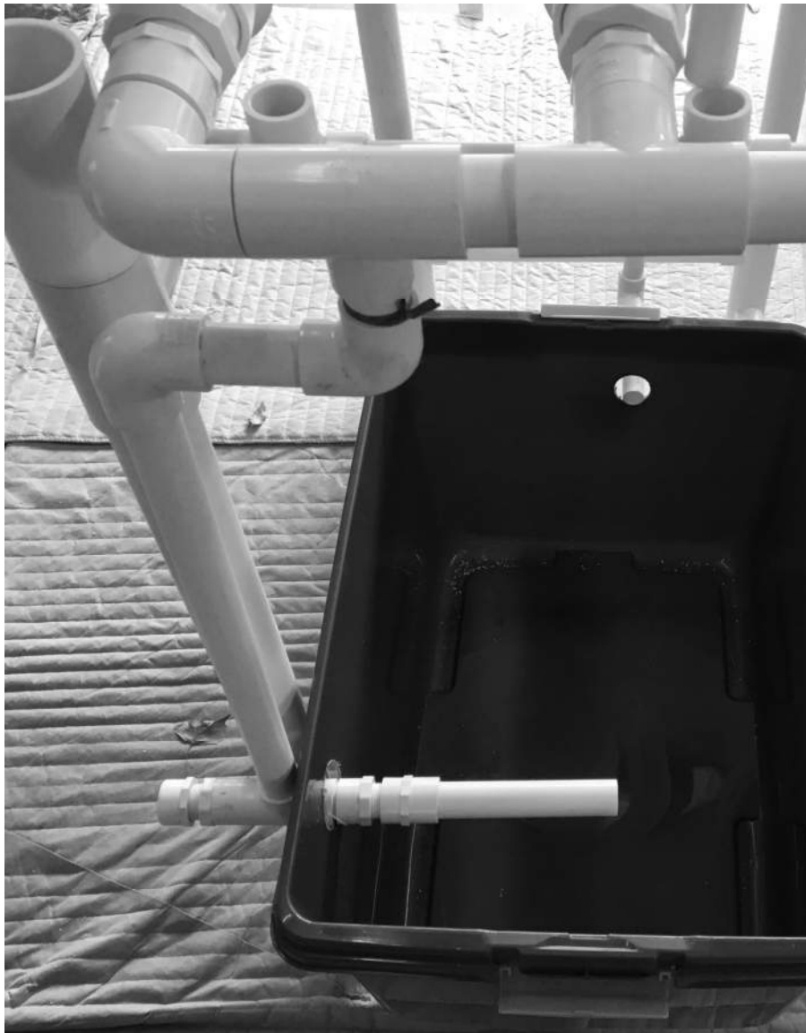
Figure 14. The irrigation to reservoir drain assembly installed. Note its Teflon tape slip connection to the underneath tee on the manifold to allow perfect vertical positioning, and the easy way to drain the nutrient solution by reversing the lower pipe segment (right, into reservoir) and cap (lower left).
