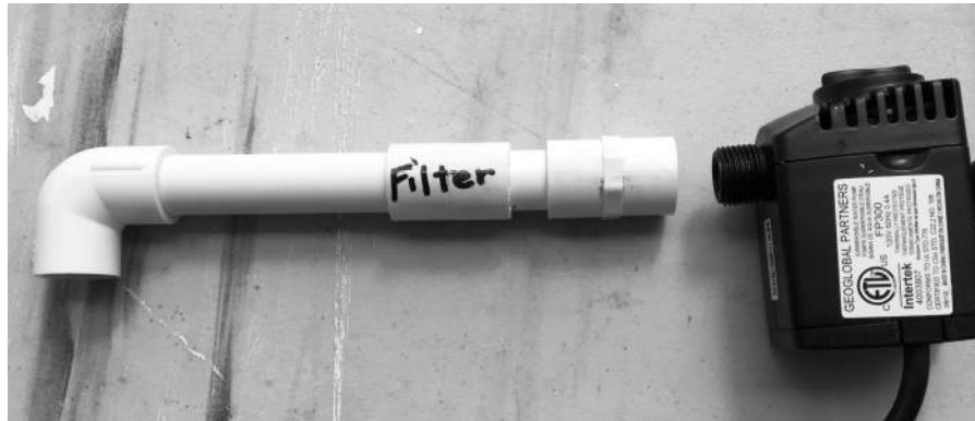
Figure 17. Pump and filter assembly. The assembly screws right into the pump. Parts are not glued to allow easy access to the filter. Filter should be checked with each nutrient change-out because particles escaping the filter will clog the spaghetti tubes. This assembly inside the reservoir connects with the drip irrigation system vertical component through the hole in the forward end of the reservoir. Some pumps have a built-in filter that's easy to check and clean. See your pump instructions.
