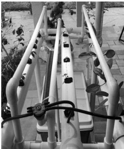
Figure 20. The plant support bars installed. To minimize unnecessary shading its not recommended installing them until plants require their support
