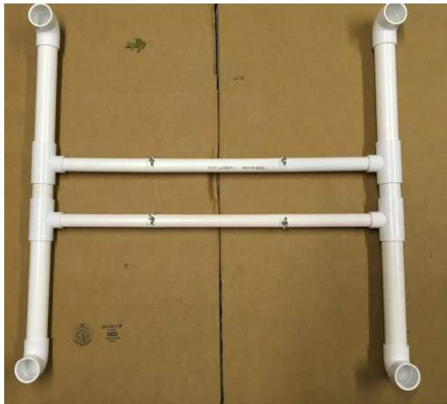
Figure 3. The Top Rack Lamp Support. Eyebolts are on the lower side and hold the lamp hooks. Shown here for the wider Indoor Garden. It will be identical but narrower for the balcony Garden.
