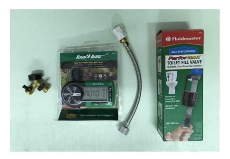
Autofill components from building (left) to outdoor Garden (right): hose bib (not shown, customer responsibility); splitter (allows Autofill to share the hose bib); timer (takes over the on/off function from the hose bib; garden hose (not shown, customer responsibility); level control valve (installed inside the Reservoir)
